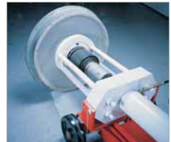
The photo above shows the Universal Puller in position on the roller bearing assembly, which is ready for removal.
