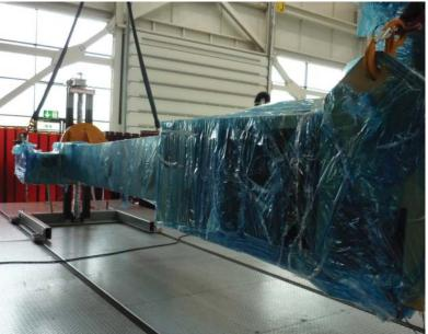
HYWEMA® developed this lifting and rotating device for welding work on frames for a manufacturer construction site vehicles. The machine is a 2-column version with а capacity of 5,000 kg and a hoisting height of 1,400 mm. The torque rating is 5.000 Nm. To enable different sizes of frames to be handled. Lift 2 is mounted on rails for easy adjustment.
