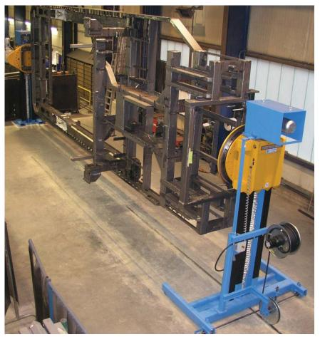
These variable installations can be used to position various different vehicle frames weighing up to 12,000 kg and having dimensions of up to 12,170 x 4,570 x 1,737 mm ergonomically and efficiently. To this end, lift no. 2 can be travelled on rails.
