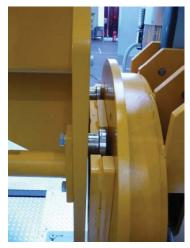
Incorporated in the turntables of each of the load supports are two slots. When the load supports have been placed in position and if the locating bolts are in the correct end positions, the adapters are secured in place by springloaded locking pins. This construction reduces retooling times considerably, which increases the efficiency rating of the unit still further.
