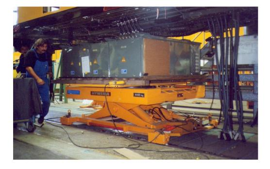
For fitting and removing drive units and powerpacks underneath railvehicles HYWEMA<sup>®</sup> developped a special hydraulic substructure fitting car model UM / FL 3, capacity 3.000 kg and modul UM /FL 5 capacity 5.000 kg.
